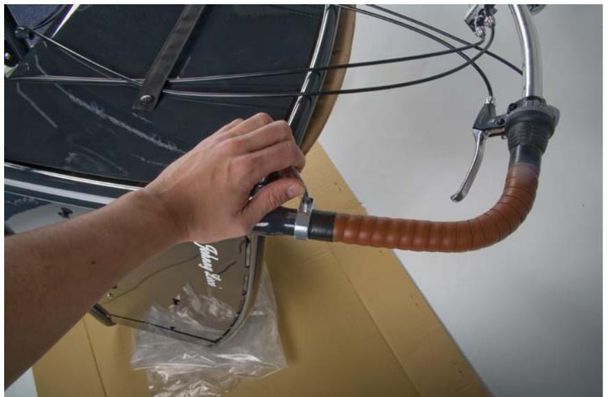
tightning handlebar clamps
