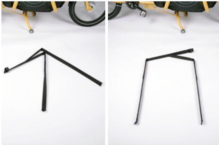
The roof frame has an extra hinge point. This hinge point makes it possible to fold the frame and store it inside the pod. When unfolding the frame secure the position with the Velcro strap
