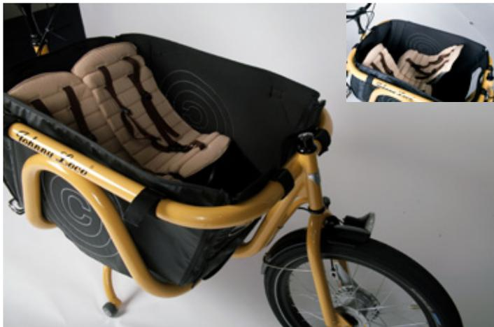
The seats can be positioned forward and backward and are able to slide backwards and forwards. When the seat are positioned opposite of each other, one facing forward and one facing backward, the shoulders of the children will not be aligned and there will be more room for taller children
