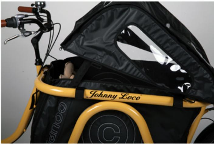
The roof can now be placed on the soft pod.
