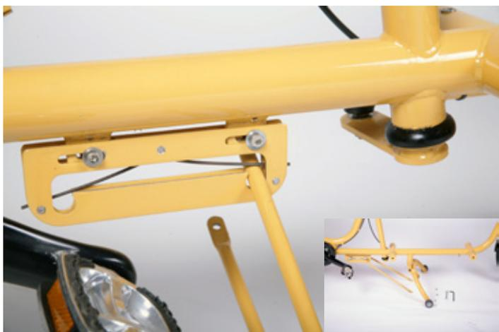
With the center tube in place, the positioning rod can be connected.
