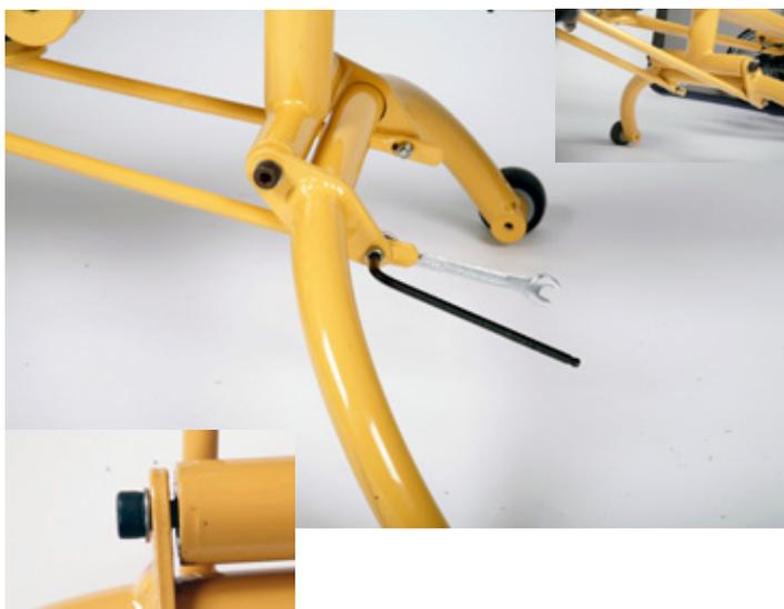
The positioning rod can now be connected to the center tube with M5 bolts and lock nuts. Make sure to put a washer between center tube and positioning rod when mounting. The bolt must not be completely tightened, leave some clearance for smooth operation
