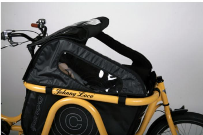
To allow the children to get out or in, both roof zippers can be undone from the front up onto the frame.
