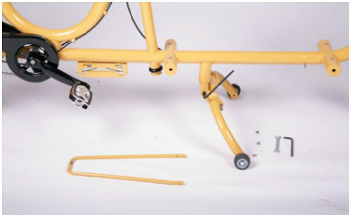
Connect the center tube of the kickstand with 2 M8 bolts to the connection tube of the frame. The bolts need to have a non threaded neck. The bolts need to be tightened completely. The non threaded part of the bolt will function as the axle of the kickstand
